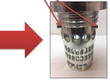
Line up one ASV tab with the centre of one of the largest holes Push down the ASV until it is flush (level) with the internal step, below the grub screw holes
