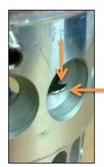
Screw the grub screws back into the device until they are flush (level) with the outside of the device
